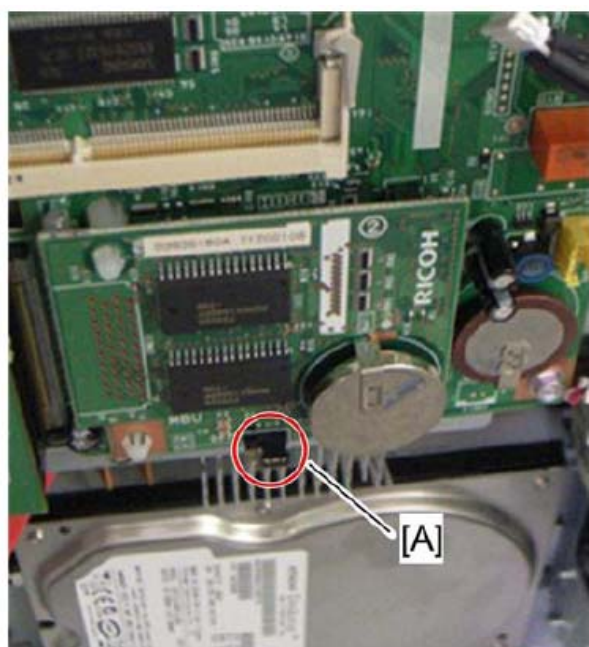
4.12 Switch the MBU battery jumper switch [A] to "ON" position.
